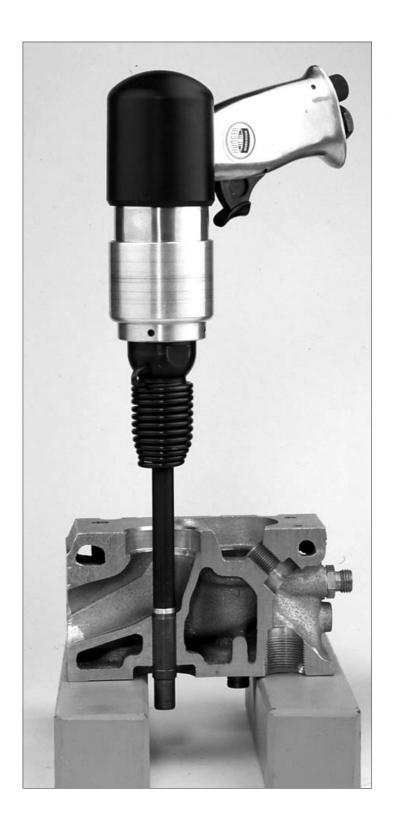
The Hunger PVM1 is designed to remove worn-out valve guides from the cylinder head and to insert new valve guides into the cylinder head.
