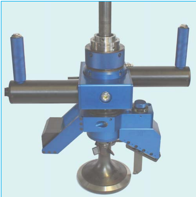
UDM4E-VK Valve Refacing Machine
